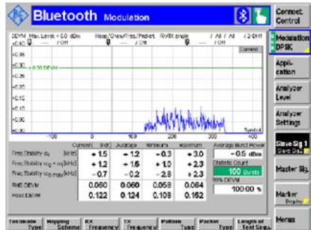
Frequency stability and modulation accuracy measurement of an EDR packet
